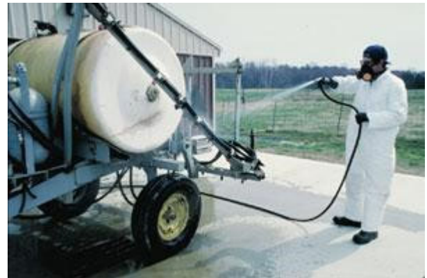
Mixing, loading, and application equipment should be cleaned and rinsed as soon as you finish a pesticide application (USDA)
