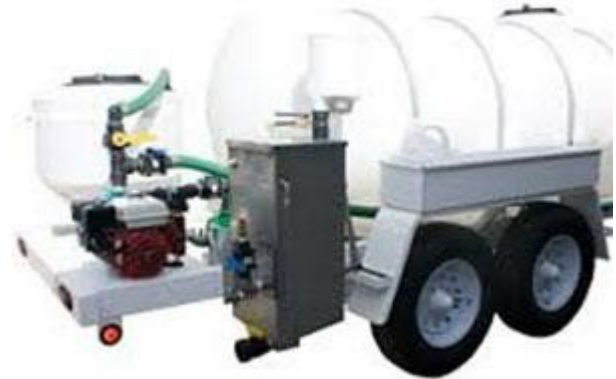
Closed pesticide mixing system (PMB Supply)
